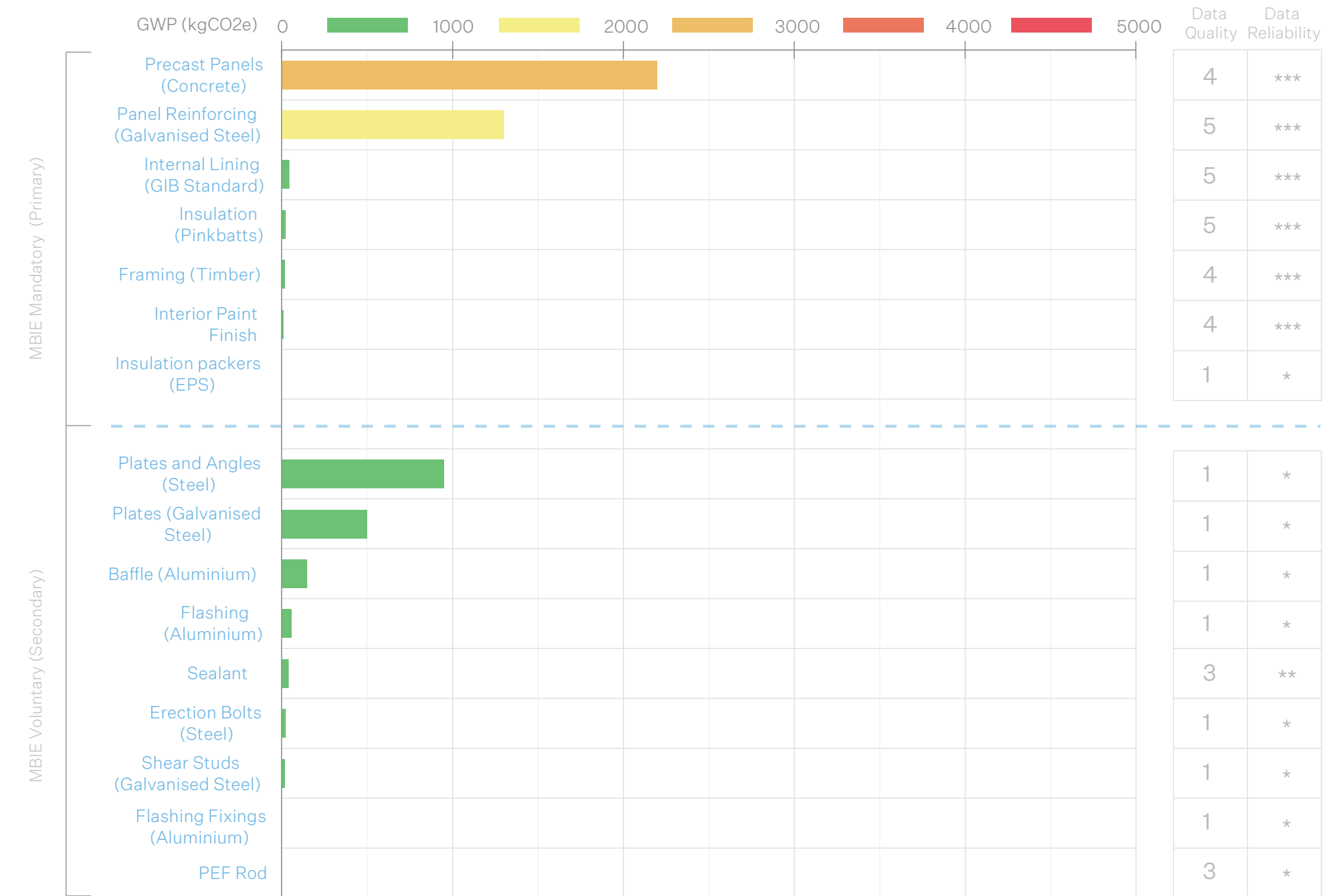
Precast Concrete Panels (FT4) Total Embodied Carbon Emissions of Facade Components per Sample Area
