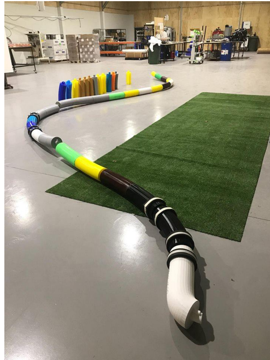
Hemo Rd Sculpture Project Rhinoceros/ Grasshopper Parametric Model. Structurally Optimised PLA Printed & Carbon Fiber Tubing Project Leads://Stacy Gordine, New Zealand Maori Arts and Crafts Institute, Te Puia Rotorua, Derek Kawiti CILOARC // GURIT Engineering // Project Manager Marc Spikerbosch & Nick Dallimore //
